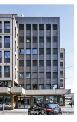
standard storeys with concrete façade elements are topped by a recessed, sheet metal-clad penthouse storey. The corner area at the junction of Hafnerstrasse and Zollstrasse is set back. This part of the building acts as a tower that goes up to the penthouse storey and is clad in sheet metal on all floors.
